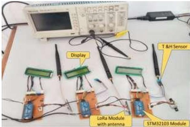
Fig. 4 LoRa system setup in lab
