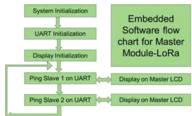
Fig.5 Master Module software flow diagram
